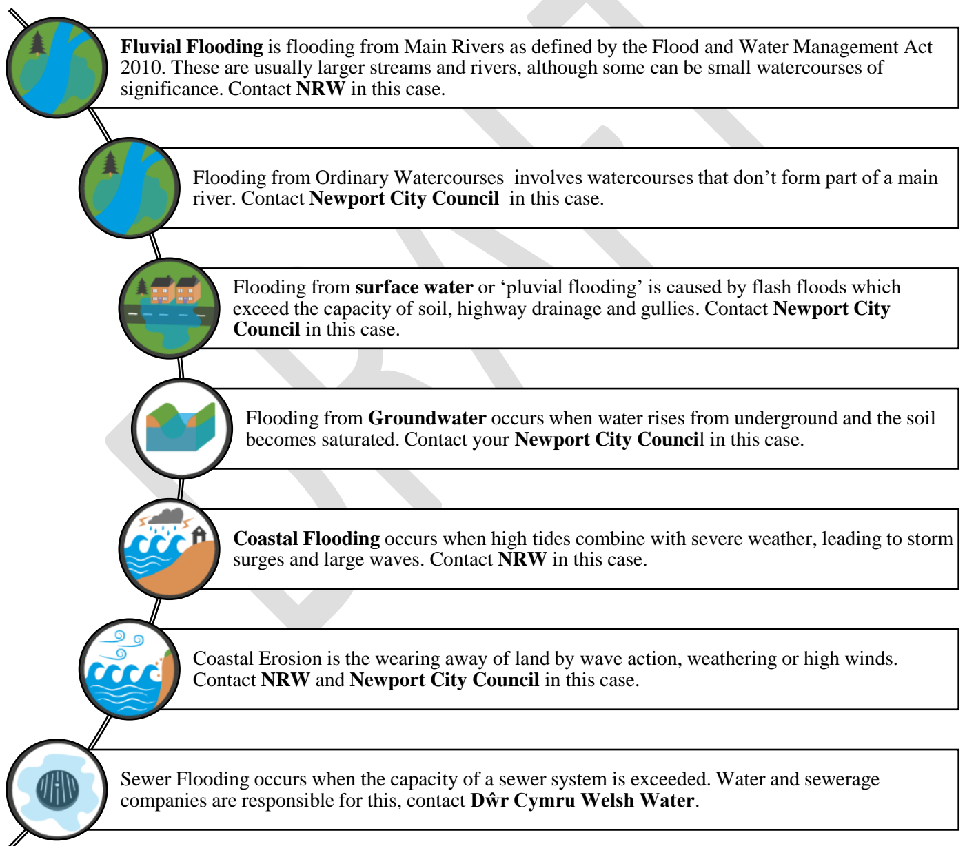
Figure 2 Sources of Flooding and responsibilities
